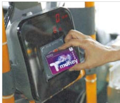
Figure 2.31 Bus card scanner attached to Seoul buses
