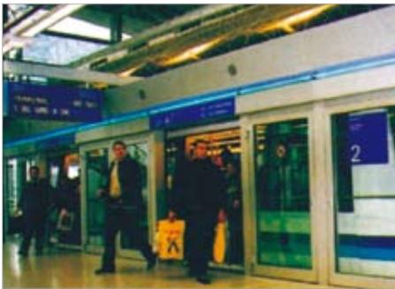
**Figure 2.6** BRT stations with horizontal entrances/exits and screen doors
